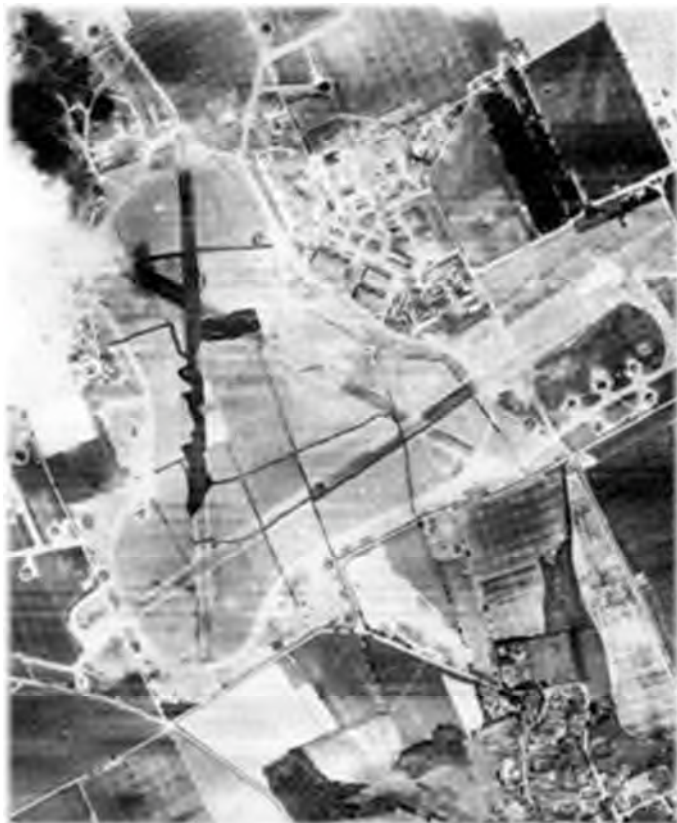
The air base Elsham Wolds: The picture is taken on 26 June 1943 from an altitude of 10.000 feet. The three runways and the hangars are clearly seen. It is a typical design of an air base for squadrons of bombers during the war. At least 17 Lancasters can be identified. The village of Elsham is seen at the bottom right corner. The geographic location between the Humber og Nene made it easy for German bombers to find the air base. During the first years of the war it was exposed to a number of bombing raids.
