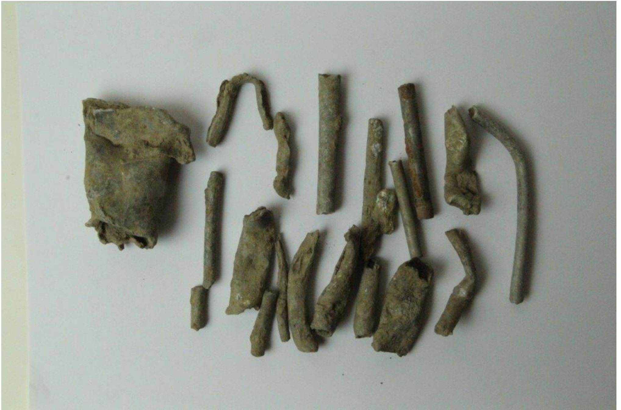
Debris field 1: Aluminium tubing (19 pieces, 150 g).
