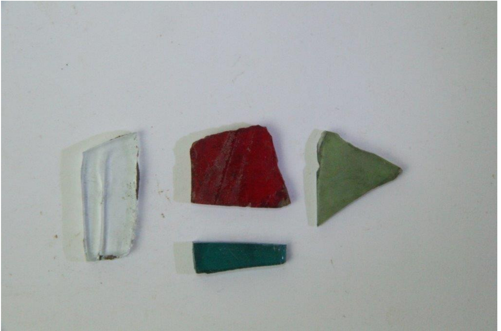
Debris field 1: Plexiglas. Red could be from the cockpit lamp. Red and green could be from the wing lights.
