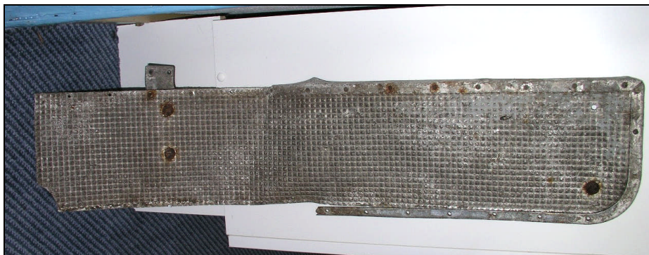
Doorstep from the Lancaster interior.
