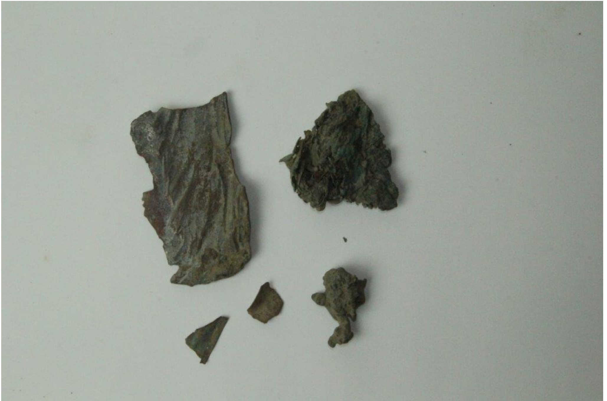
Vragdelsfelt 1: Smeltet kobber.
